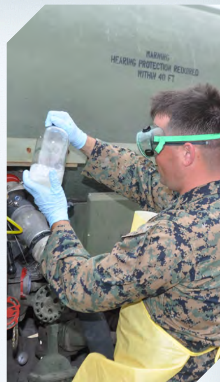
Marine Corps Sgt. Andrew Grable examines a sample of fuel before conducting laboratory testing to ensure it meets military specifications. The Marines tested a prototype Expeditionary Mobile Fuel Additization Capability during the Rim of the Pacific exercise.
